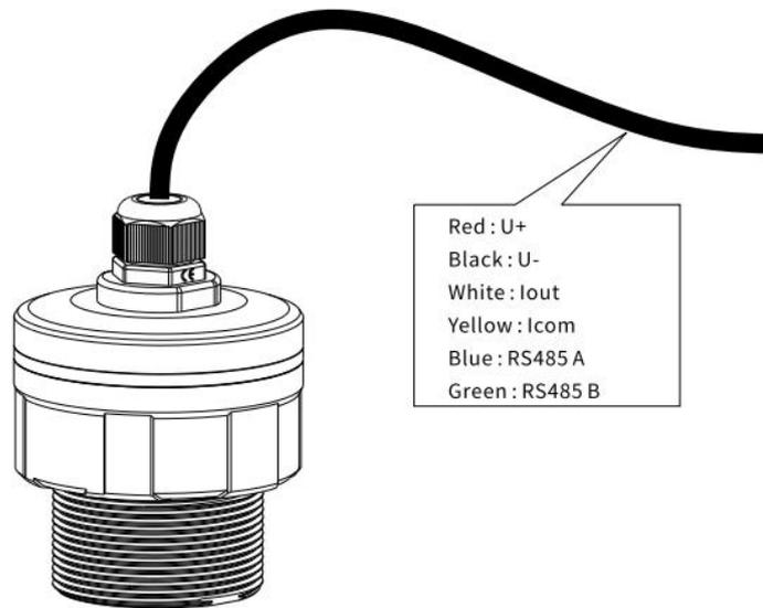
Figure2 Diagram of 4-wire cable
