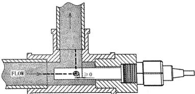
Wrong: An air dead space is formed in the upper part of the pipeline. Although the opening of the conductivity cell affects FLOW, there is still no fluid flowing through the conductivity cell, and the measurement data is worthless and unstable.
