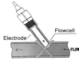
Right: part of the flow flows through the waist hole of the conductivity cell and is constantly updated, and the measurement data is correct and stable and true.
