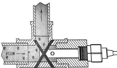
Right: part of the fluid in the pipeline flows through the conductivity cell and is constantly updated, so the measurement is accurate, and the opening of the sensor must face FLOW.
