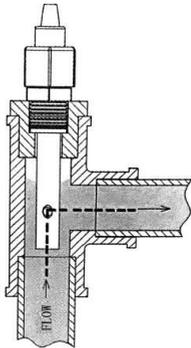
Wrong: The water flow in the pipeline cannot be guaranteed to be full, and the discharged water flow will form higher gas accumulation, the conductivity cell constant is an unknown number, and the data is invalid and unstable.
