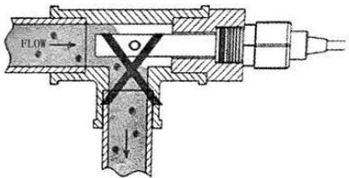
Wrong: The water flow of the conductivity cell installed in the angular direction cannot flow through the waist hole, and the gas inside the conductivity cell causes the measurement value to be invalid and very unstable.
