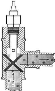
Right: The waist hole of the conductivity cell is located in the fluid, and part of the fluid flows through the conductivity cell to be continuously updated, and the measurement is accurate.
