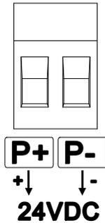
The chart recorder provides an output of 24V, 60mA.
