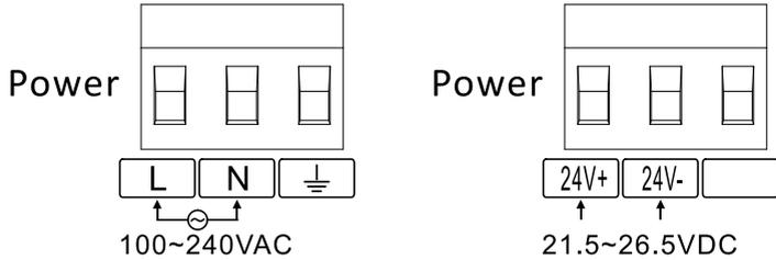
According to the chart recorder model, select 220VAC or 24 VDC wiring.
