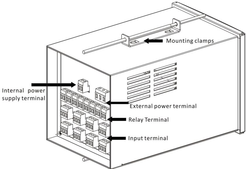
Power supply terminal; mounting clamps; external power terminal; relay terminal; input terminal
