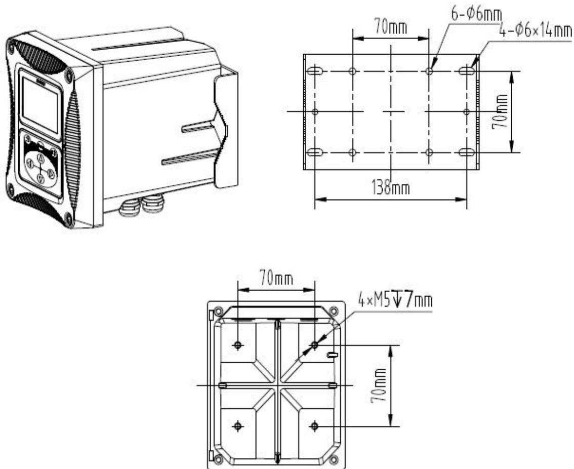
Figure 3 Installation Size
