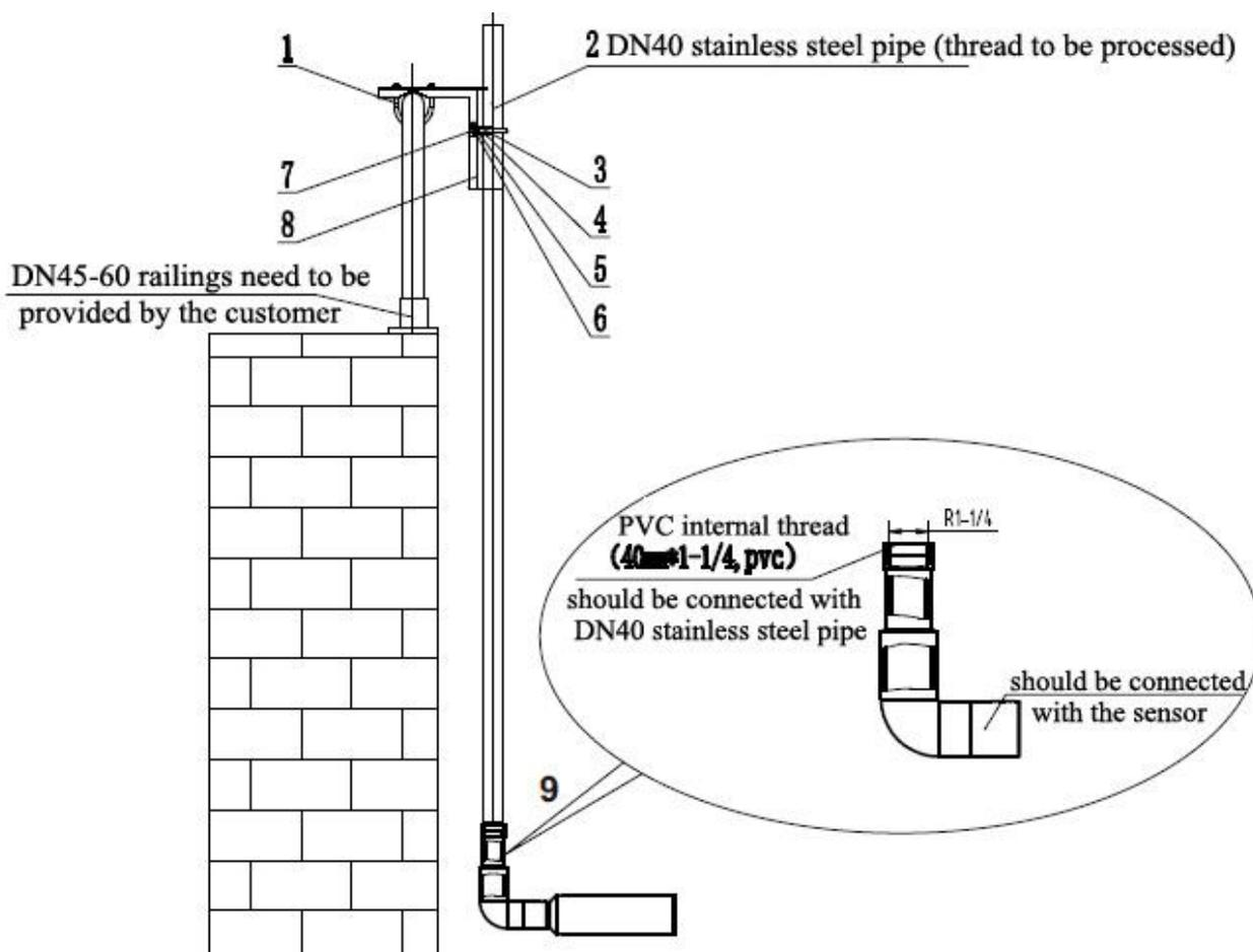
**Figure 11 Schematic Diagram on the Installation of Sensor**
