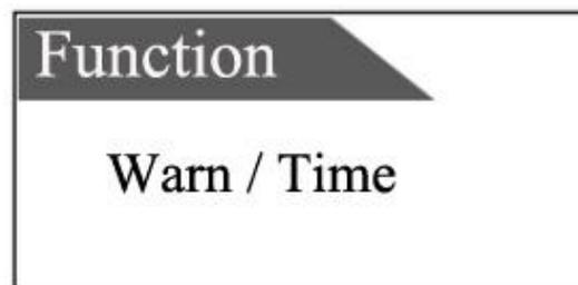
**Time:**The function of relay's timing is, it works in a specific period of time, which is set as "Keeping", while in the rest of time, it's closed, and the time is a designed period. If you want the relay to work for 10s, closed for 50s, then you can set the "Keeping" as 1min.
