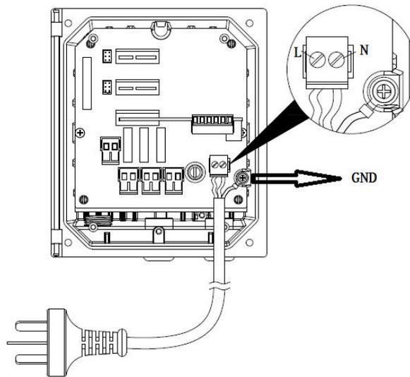
**Figure 8 AC220V Power Supply Wiring**
