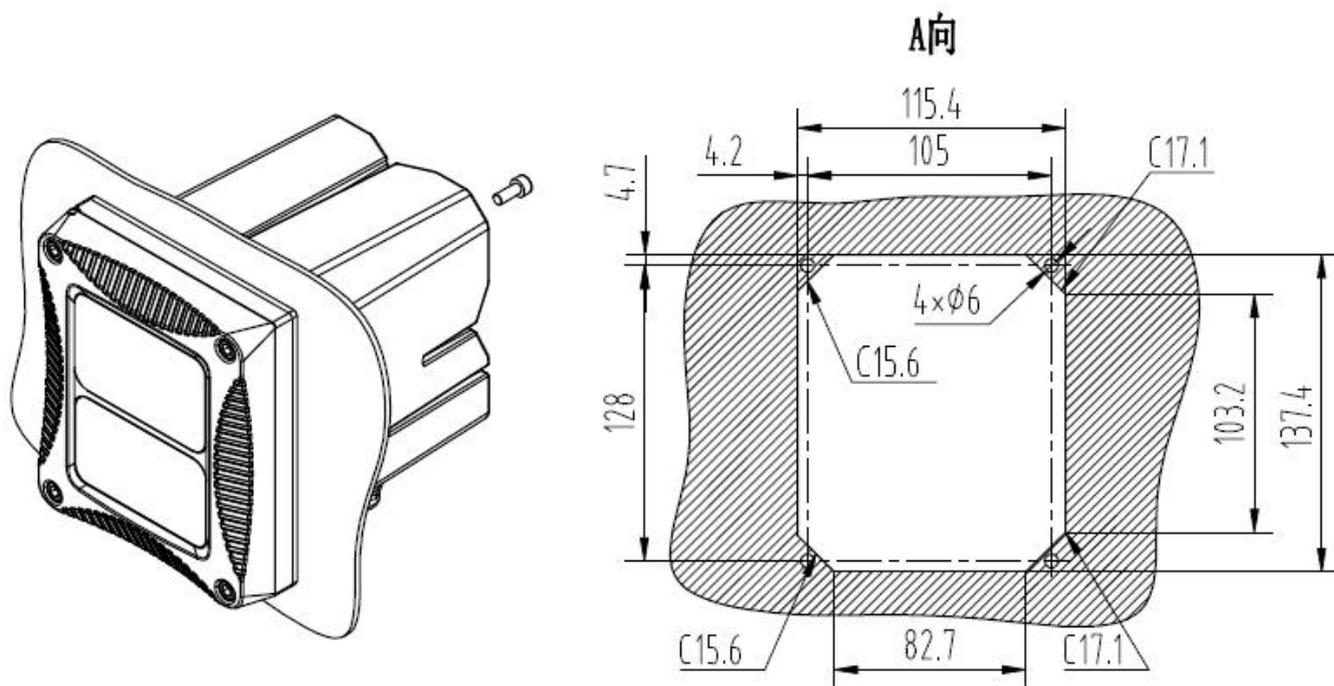
Figure 5 Panel Installation
