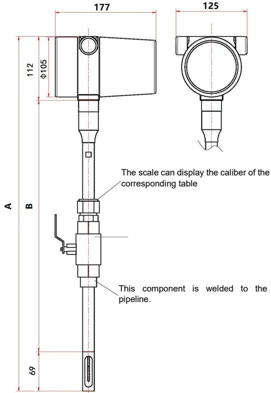
Fig.2 Insertion flow meter (Unit: mm)
