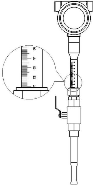
Fig.1 Standard Insertion Flow Meter
