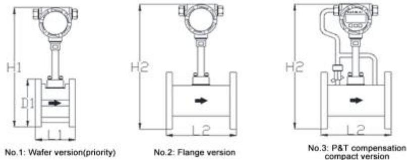
SUP-LUGB-B Vortex flow meter max configuration size table (unit: mm)
