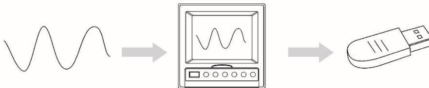
The data that have been saved to an external storage medium can be displayed on a PC using the standard software that comes with the package.
