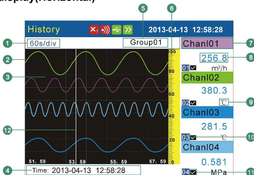
1. Trend cycle. Each grid means the length. The cycle is related with saving interval, Time length = saving interval × Zoom multiple × 30.
