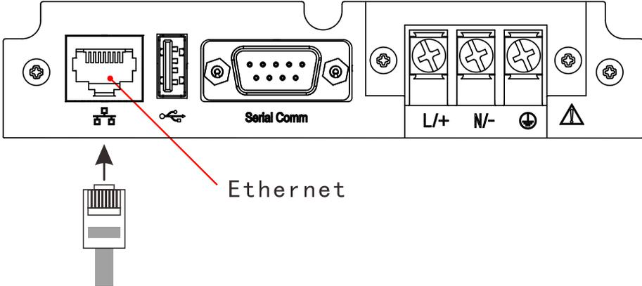
Use network cable connector to connect RJ45 connector.
