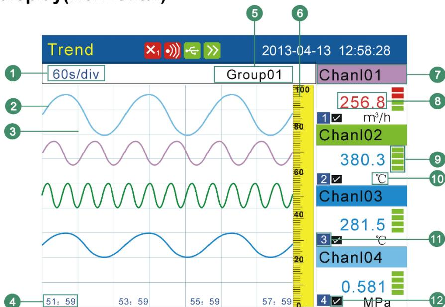
1. Trend cycle. Each grid means the length. The cycle is related with saving interval, each grid time length = saving interval × 30.
