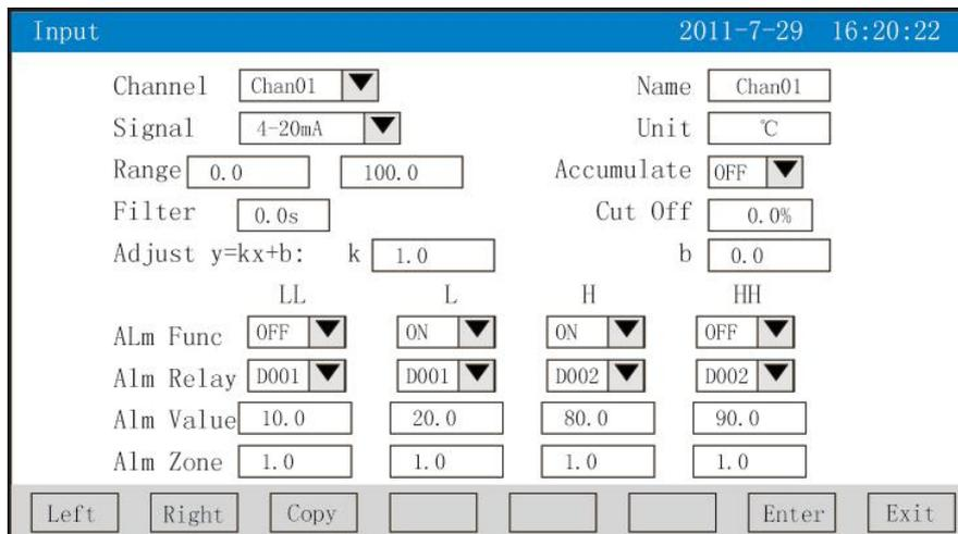
\* Configuration channel: choose the channel number of the display configuration
