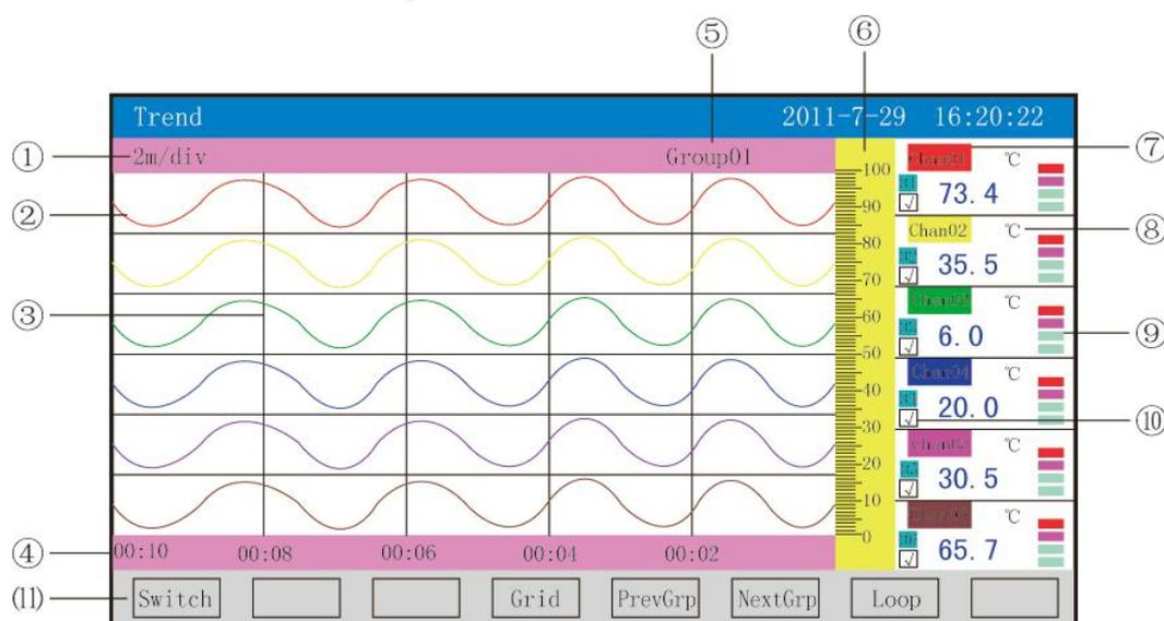
①: Time scale: It means the length of time per grid and the time scale is related to the recording interval, as shown in the table below:
