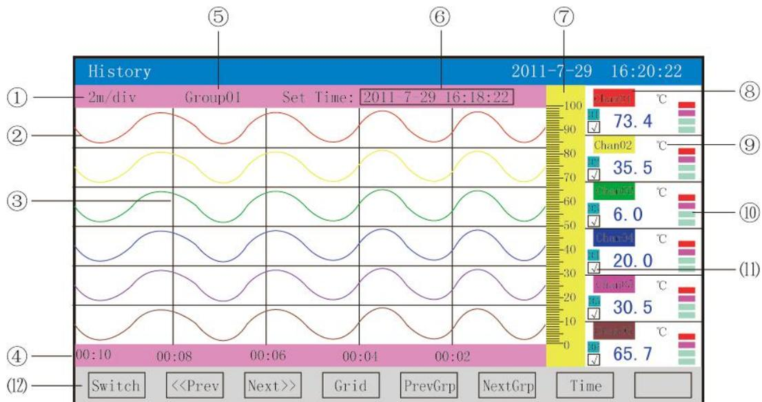
①: Time scale: It means the length of time per grid and the time scale is related to the recording interval. Please refer to the instruction described in 4.3 Real-time Curve Menu for details.
