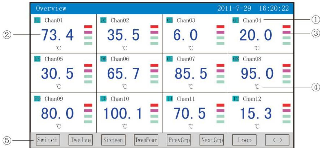
①: Channel name: It means the corresponding project bit number of each channel and can be set. (Please refer to 4.12.4.1 Input Method of Channel Bit Number for the setting method.)
