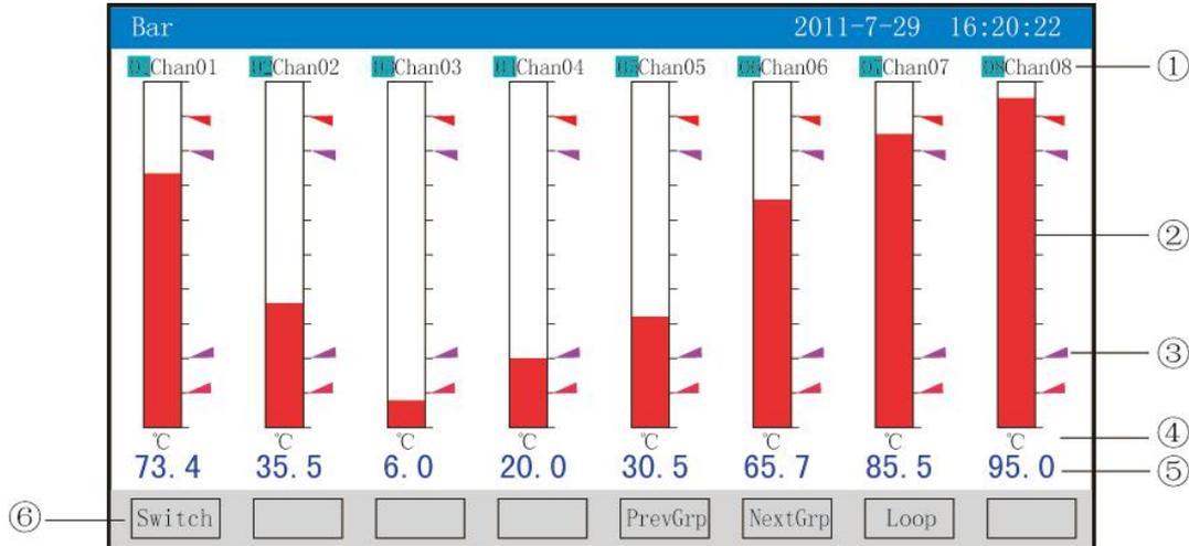
①: Channel name: It means the corresponding project bit number of each channel and can be set. (Please refer to 4.12.4.1 Input Method of Channel Bit Number for the setting method.)
