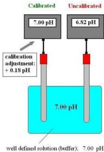
To achieve the best possible accuracy, the calibration should cover the range of the desired measurement values. If the readings go beyond the calibrated range, the pH meter assumes linearity and simply extrapolates the value to be displayed. The true value may be slightly different.
