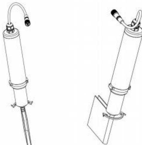
Fig.13 Polishing of Membraneless Dual Platinum Ring sensor
