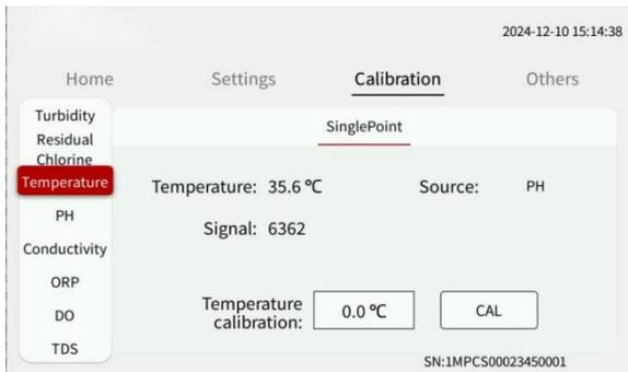
Fig.10 Temperature Calibration Display Diagram
