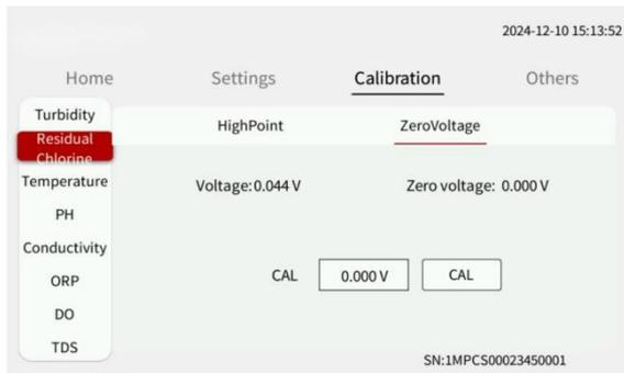
Fig.9 Display of Zero Calibration
