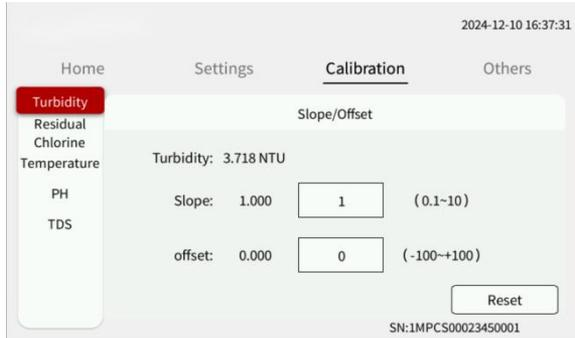
Fig.7 Calibration Diagram for Slope and offse
