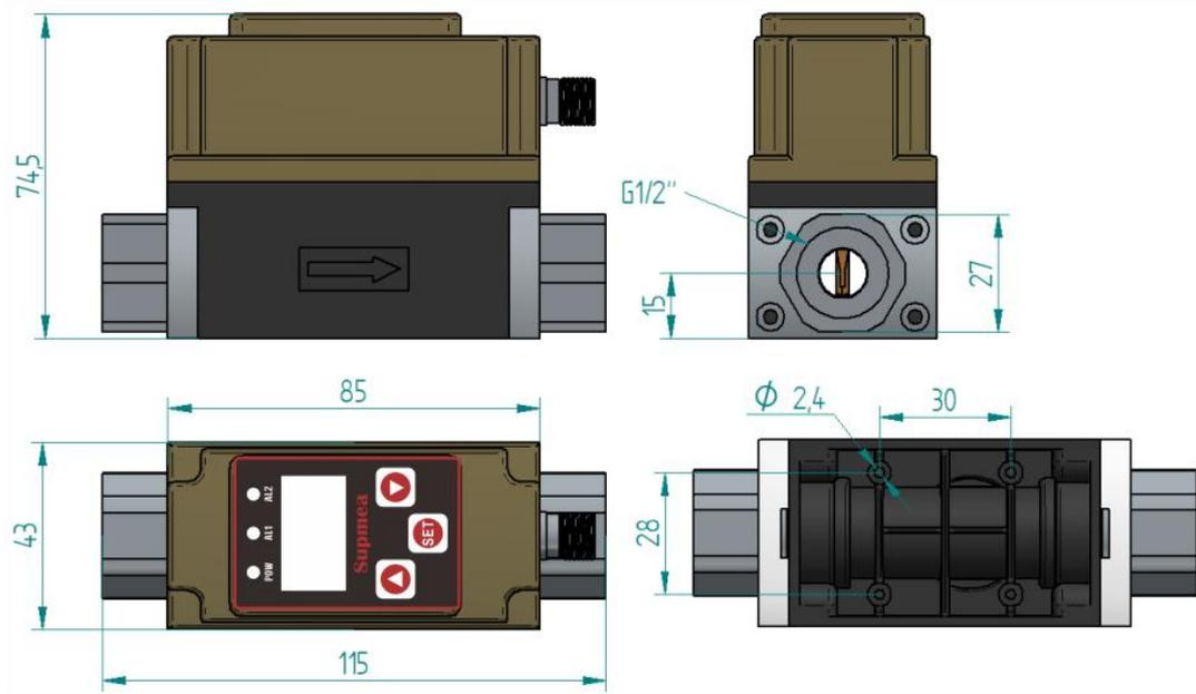
Figure 5 Product Dimensional Drawing (Unit: mm)
