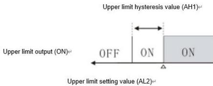
★Bit-type upper limit alarm output:
